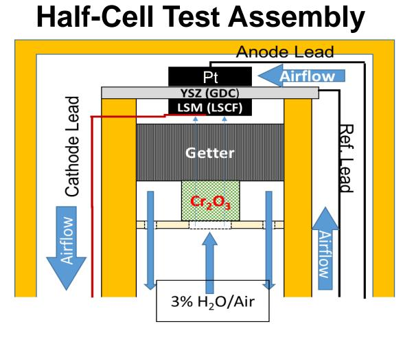
SOFC Accelerated degradation testing with pure  $Cr_2O_3$  pellets and a flow rate of 150 sccm in a 1" tube.
