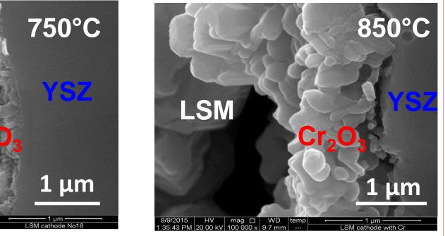
**SEM images** show that the thickness of Cr<sub>2</sub>O<sub>3</sub> layer in the LSMIYSZIPt cells increases with operating temperature.
