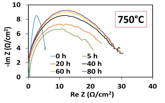
Cell polarization resistance (Rp) increases with time.
