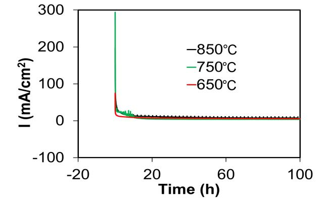
LSMIYSZIPt cells degraded rapidly in Cr containing air.
